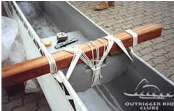
'iako to wae and mo'o showing other important tools - tape measure, level, and line wax
