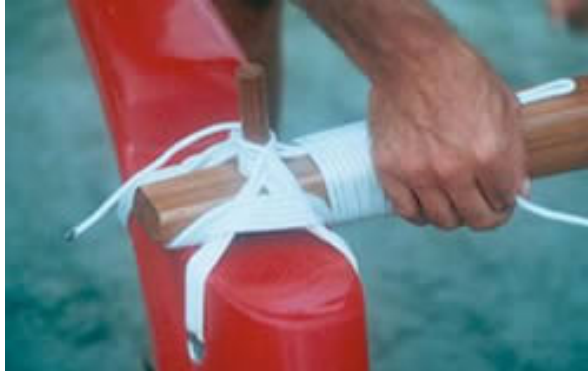
'iako to ama showing a clean and strong connection in the final wrapping and knot
